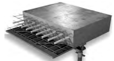
Figure 12 : Plancher solaire direct.
